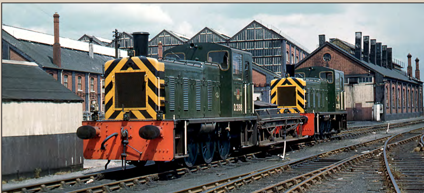
Below: With a Great Western Railway 'shunters truck' coupled between, two of the Swindon-allocated 'standard' small 0-6-0s Nos. D2188 and D2189 pose in Swindon Works yard in October 1960. When the early examples of the fleet emerged from Swindon they were fitted with a non-screw three link coupling, later examples had the screw design. www.colour-rail.com
