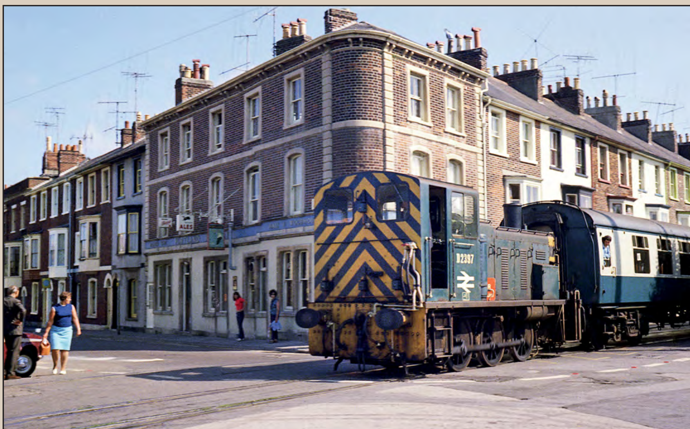
Below: With heads turning to see the unusual sight of a train running along the public streets of Weymouth, Rail Blue No. D2397, a dual-brake fitted loco runs between Weymouth Quay and town station with a through train to London Waterloo in the early 1970s. In the summer season two through trains operated each day; after the '03s' were retired, modified Class 33/1s with plug-in warning bells/flashing lights were introduced. www.rail-online.co.uk
