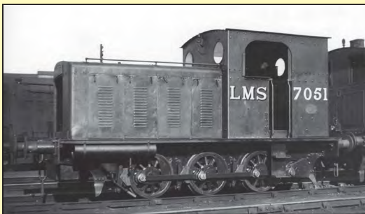
Above and Below: Hunslet Engine Co built LMS No. 7401 in 1933, it was later renumbered to 7051. This prototype was powered by a 150hp (111.8kW) MAN 6-cylinder engine powering a mechanical transmission. Like many of the early diesels, No. 7051 went into War Department use in 1940 working at Capenhurst, before returning briefly to the LMS the following year, before going back to War Department use in 1944-45. In December 1945 the loco was sold back to its builders. Both: CJM-C
