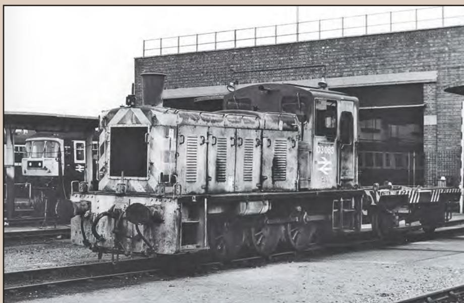
Left: One of the problems of continually operating a locomotive through the carriage washing plant, especially if it was using strong bleach, was that after a time the loco became faded and almost white. By the look of the paint work, this was the problem with No. 03063 seen stabled at Hull Botanic Gardens depot in summer 1980. This loco after withdrawal was preserved and is currently on the North Norfolk Railway at Sheringham. CJM
