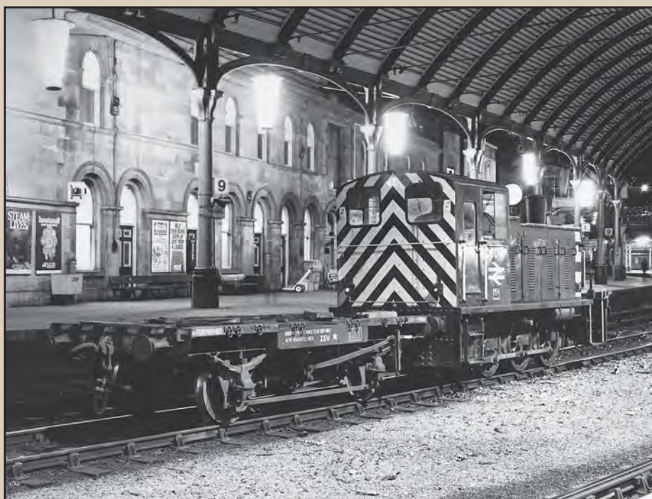
Above and Right: For many years in the 1970s and 1980s, a single Class 03 attached to a shunting match wagon, coupled to assist in the positive operation of track circuit equipment, was frequently to be found stabled on the through siding tracks in Newcastle Central station, from where they carried out shunting of van trains within station limits especially during the evening and overnight. These two views show vacuum-brake fitted No. 03079 coupled to shunting truck TDB701983 stabled in the small hours of 20 May 1982. Both: CJM
