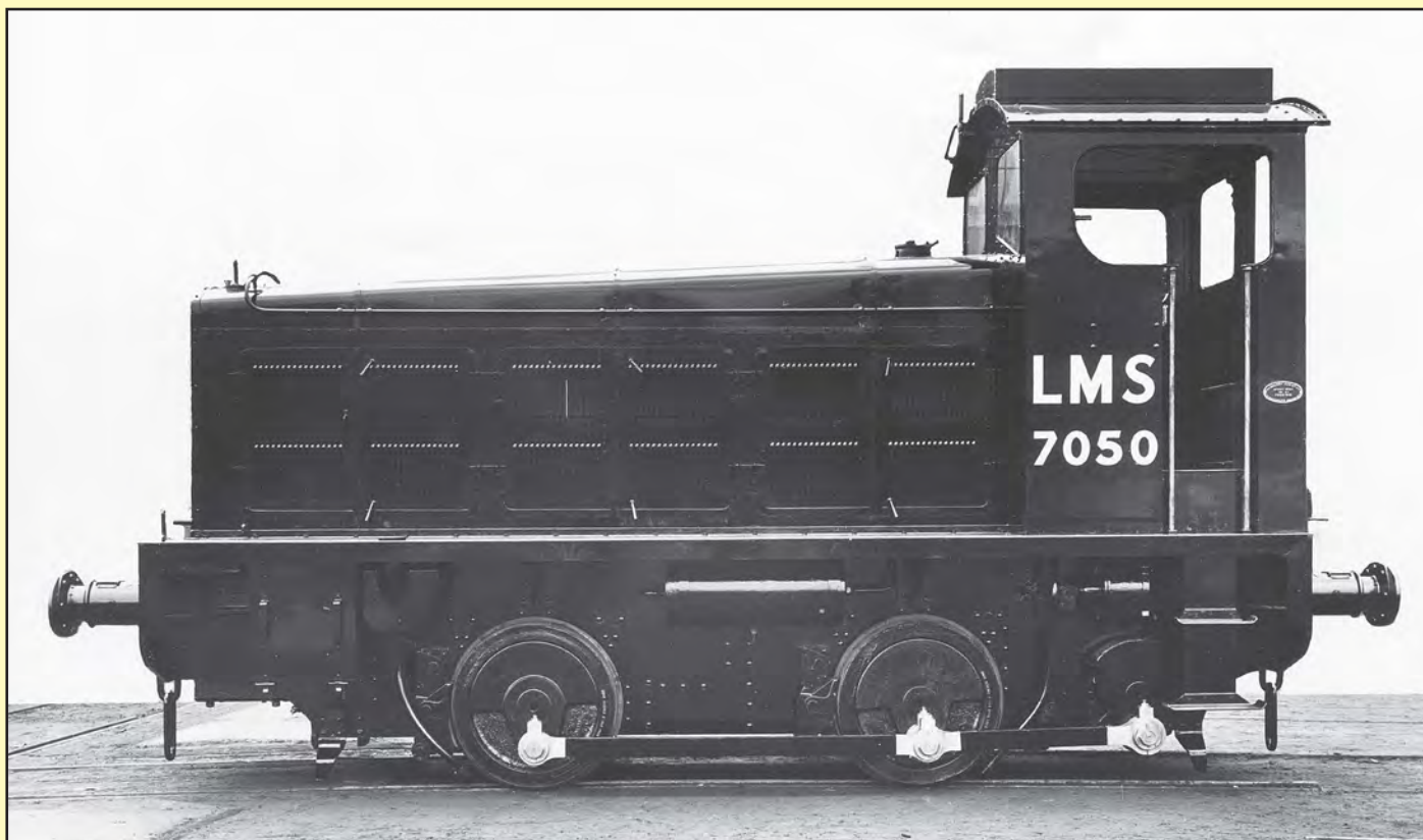
Above: The rather pleasing tapered bonnet design of LMS No. 7050, built by Drewry Car at the Dick Kerr Works in Preston is clearly shown in this view. After initial trials in the Preston area, the loco was sold to the LMS. After a few years the central raised section of the cab roof was removed. In 1943 the loco was transferred to the War Department, later working for the Ministry of Defence. After withdrawal the loco was preserved and is now part of the National Collection, based at York CJM-C
