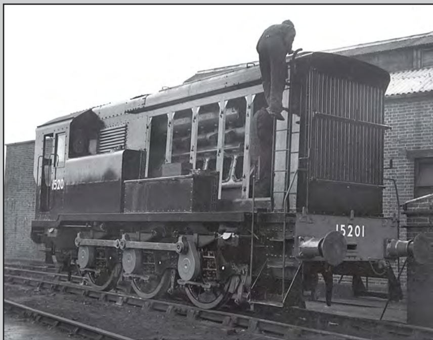
Above: In 1937 the Southern Railway took delivery of three 'standard' design 0-6-0s fitted with the EE 6K engine. The first of the fleet Southern 1 is seen in as built condition painted in black livery before entering service at Norwood. CJM-C
