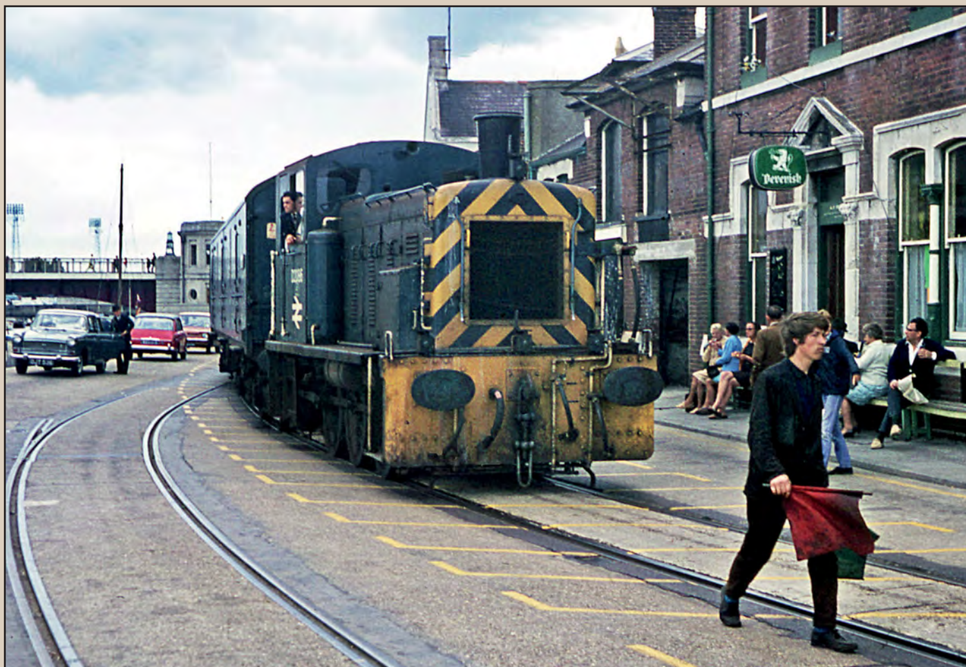
Above: For many years after the demise of steam traction powering trains along the Weymouth Tramway line between Weymouth station and Quay, Class 03s were the preferred power. As most of the Southern Region stock used on these services were air brake fitted, dual brake locos were required. DB fitted No. D2086, complete with high level duplicate air pipes, traverses the quay line on 1 September 1970. As these trains operated along the public street, a man had to walk in front with a flag, protecting cross-traffic and ensuring cars, bikes and people were clear of the tracks. www.colour-rail.com / M. H. Yardley
