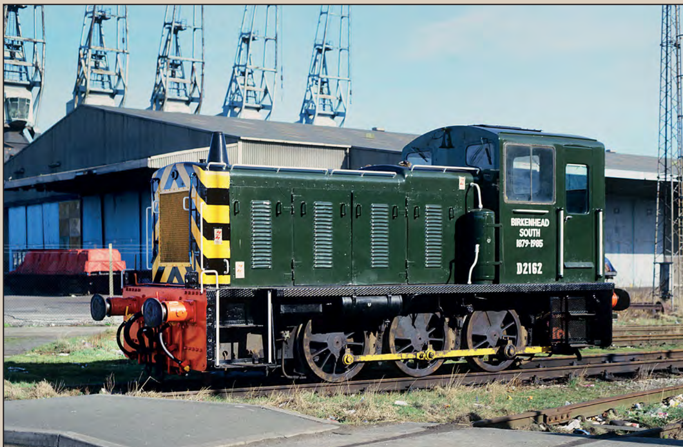
Above: No. 03162, the original D2162, was restored to 1960s BR green livery in January 1987 by staff at Birkenhead South depot, to mark the closure of the depot. In addition to green livery, the loco was named Birkenhead South 1879-1985, reverting to its original 'D' prefix number. The as built 'flower-pot' style exhaust stack was replaced with a short conical type. The dual brake fitted loco is seen in immaculate condition at Birkenhead Docks on 28 February 1987. After withdrawal in March 1989, this loco entered preservation and is currently at the Llangollen Railway. CJM
