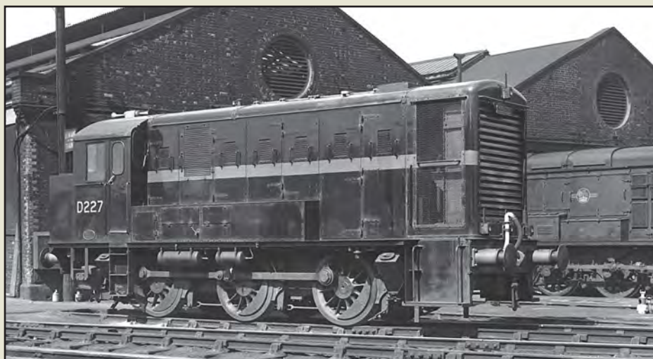
Left: Painted in a very attractive black livery off-set by an orange bodyside band and down pointing nose chevron, the diesel-hydraulic member of the EE demonstration pair No. D227 is seen at Stratford depot. This loco used a Krupp 3-D-46 transmission, allowing 330hp (246kW) power at the wheel. The prime mover was a standard English Electric 6K, but set to deliver 500hp (373kW). CJM-C
