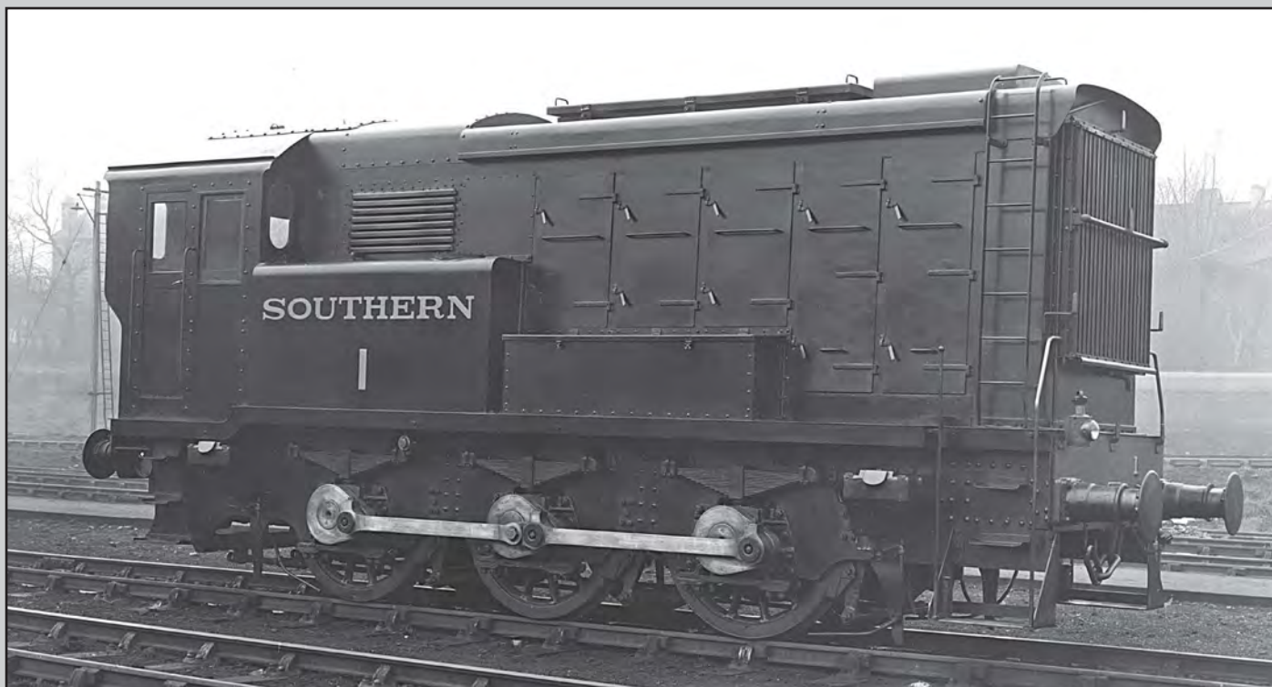
Above: In 1937 the Southern Railway took delivery of three 'standard' design 0-6-0s fitted with the EE 6K engine. The first of the fleet Southern 1 is seen in as built condition painted in black livery before entering service at Norwood. CJM-C
