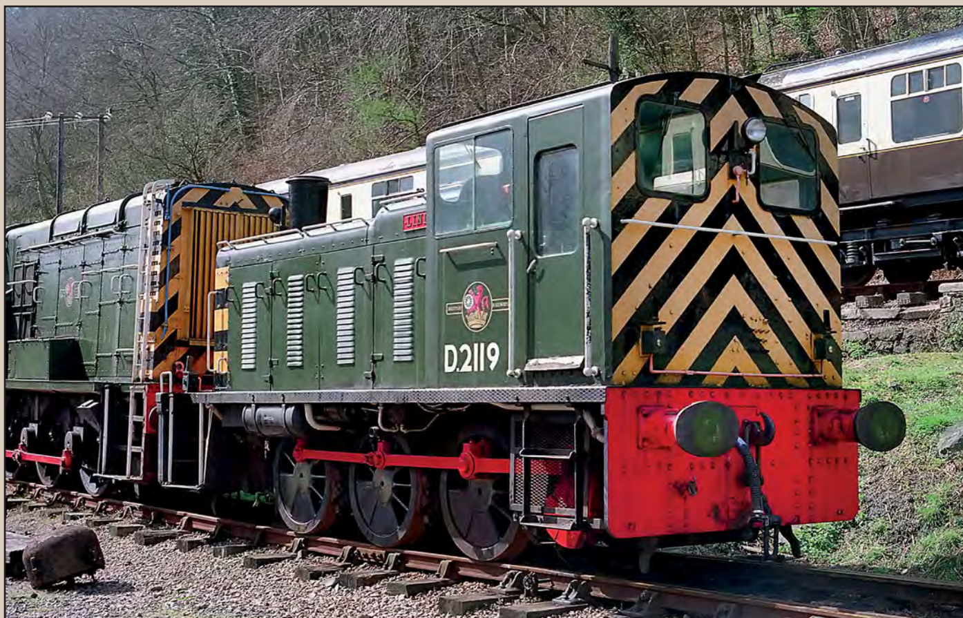
Above: One of the Class 03s which received a reduced height cab structure for operation over the BPGV line in West Wales, No. D2119 (03119) is now preserved. In this 4 April 1994 view, the loco is seen restored to 1960s BR Green livery with wasp warning ends, carrying the cast name Linda, at Norchard on the Dean Forest Railway. This loco later went to the West Somerset Railway (March 1996) and is now kept at the Epping & Ongar Railway. dieselimagegallery.com/ Jim Binnie
