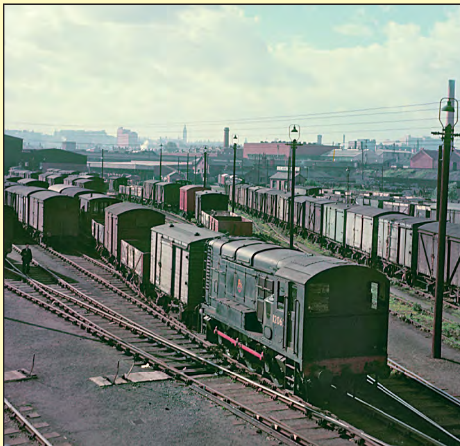
Above: The result of all the trial operations of various LMS shunting loco designs, saw the final refinement of the design which resulted in the forerunner to the standard 'large' UK 0-6-0 loco, later classified as Class 08 and 09. The 1944-LMS 'standard' shunter emerged in 1945 when LMS 7120 was rolled out of Derby Works, construction was slow and by the time of Nationalisation in January 1948 only 12 locos had been delivered carrying LMS numbers, the remaining locos emerged under BTC control and took the five-digit 12045-12138 numeric sequence. LMS No. 7120 was later renumbered as BR No. 12033. Members of this class, which were technically different from the later 'standard' design, were classified under TOPS as Class 11. CJM-C
