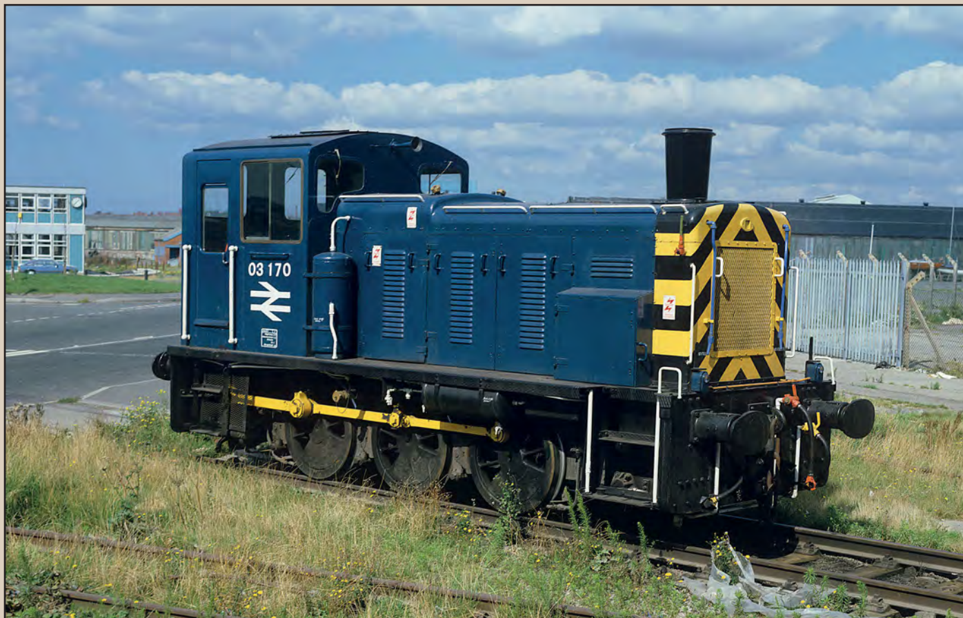
Below: With slightly thinner numbers than standard, No. 03170, another of the dual brake locos, stands between duties at Birkenhead Docks on 28 February 1987. In those days the '03s' working within the dock complex were left all weekends stabled around the yard, with no fear of damage or 'repainting' by vandals. This image clearly shows the extra box fitted to the frame of dual brake examples. This was a hinged door housing access to the air compressor. This loco was withdrawn from Birkenhead in March 1989 and is now preserved at the Epping & Ongar Railway. CJM
