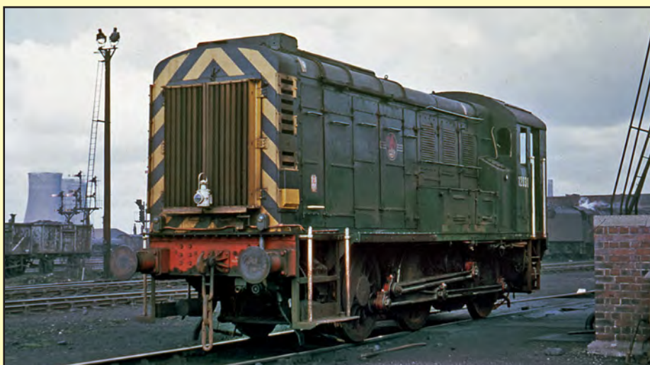
Above: After warning ends became the norm on 'modern traction' many of the remaining 'jackshaft' 0-6-0s were given yellow-black 'wasp' ends, as shown on No. 12009, displaying tatty BR green livery and the Lion holding the Wheel motif on the bodyside at Speke on 16 March 1968 after withdrawal. www.colour-rail.com
