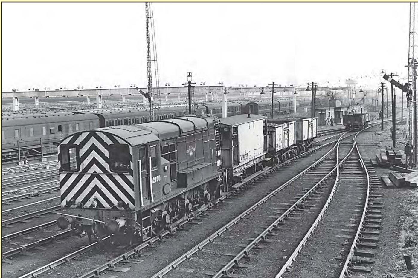
Above: As part of BR policy of the era, the LMS-design 'standard' 0-6-0 shunting locos obtained 'wasp' yellow/black warning end from the mid 1960s. Here, No. 12100 pushes wagons over the hump at Willlesden. This loco shows standard BR green livery. No. 12100 was introduced in April 1952 allocated to Derby and was withdrawn from Springs Branch, Wigan in March 1969. CJM
