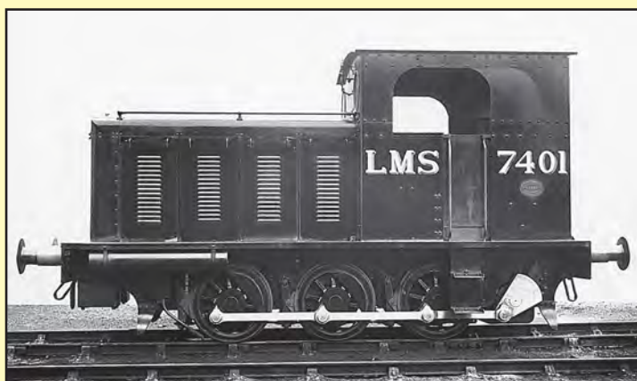
Above and Below: Hunslet Engine Co built LMS No. 7401 in 1933, it was later renumbered to 7051. This prototype was powered by a 150hp (111.8kW) MAN 6-cylinder engine powering a mechanical transmission. Like many of the early diesels, No. 7051 went into War Department use in 1940 working at Capenhurst, before returning briefly to the LMS the following year, before going back to War Department use in 1944-45. In December 1945 the loco was sold back to its builders. Both: CJM-C
