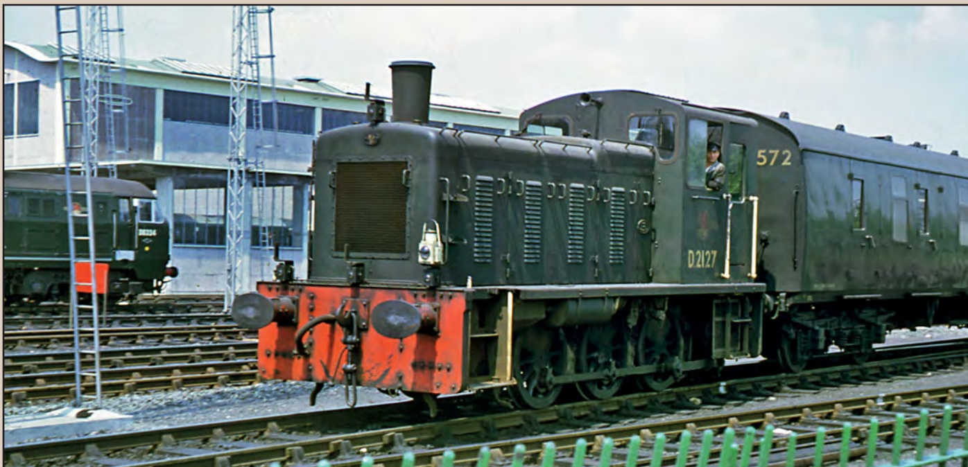
Above: Introduced in December 1959 as a product from Swindon Works, No. D2127 was first allocated to Swansea, but by the following year was transferred to the West Country and worked from Laira depot in Plymouth for several years. On 9 June 1962 the loco is seen shunting a BR Southern passenger coach at Laira depot, while a NBL Type 2 is seen in the background. This loco was one of the early withdrawals being taken out of service in May 1968. www.colour-rail.com
