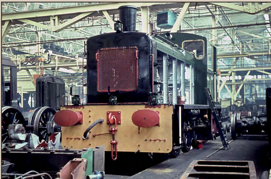
Left Top: With its first coat of green paint applied, No. D2175 is seen in advanced stage of construction at Swindon 'A' shop on 3 December 1961. This loco was destined for the Southern Region at Ashford, Kent when delivered towards the end of the month. Records show that at the height of the standard small shunting loco assembly project, Swindon had as many as 20 locos in various stages of assembly at one time. www.colour-rail.com
