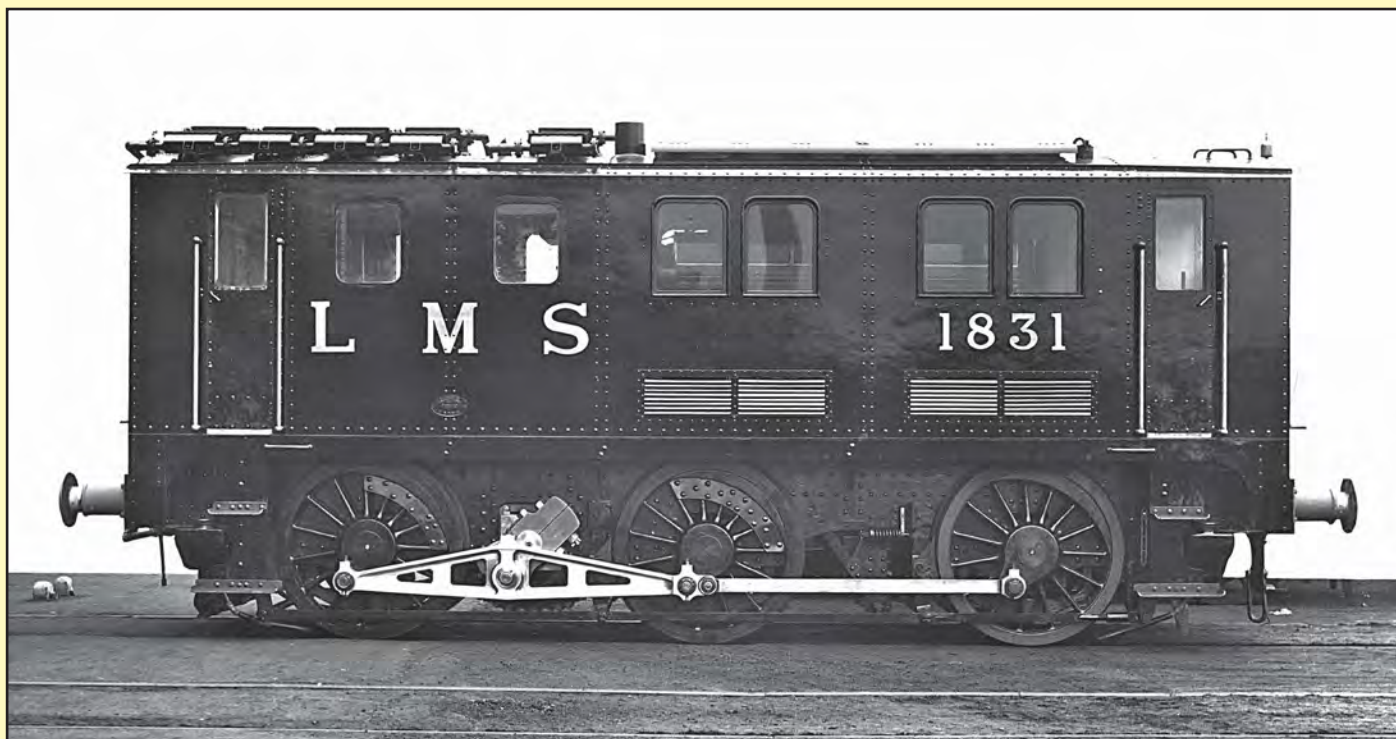
Above: Recorded in October 1932, LMS pioneer 0-6-0 diesel-hydraulic shunting locomotive No. 1831 is seen in as built condition at Derby. The locos No. 1 or main cab is seen to the left. Built on the frame of withdrawn Johnson Class 1F steam loco, from which it took its number, the 'new' diesel was powered by a 400hp (298kW) Paxman engine. CJM-C
