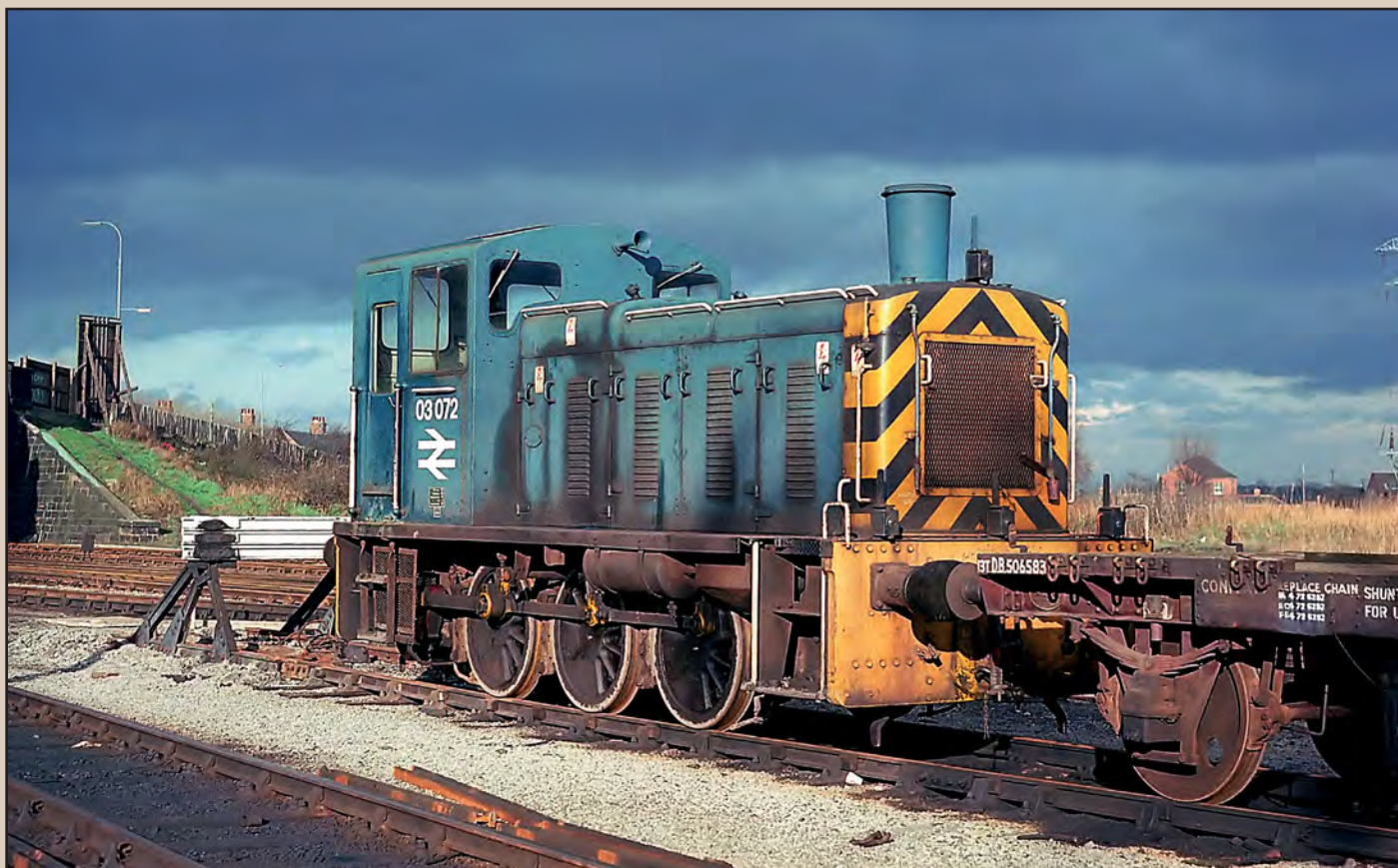
Above: Under a very stormy sky, Class 03 No. 03072, painted in mid-1960s Rail Blue, takes rest between duties at Darlington on 12 March 1978. This image clearly shows the single tube warning horn, mounted at cant rail height on the front of the cab. No horn was provided on the cab end. dieselimagegallery.com / Jim Binnie
