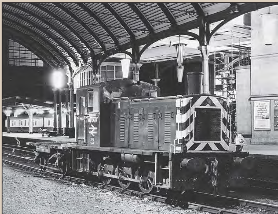
Above and Right: For many years in the 1970s and 1980s, a single Class 03 attached to a shunting match wagon, coupled to assist in the positive operation of track circuit equipment, was frequently to be found stabled on the through siding tracks in Newcastle Central station, from where they carried out shunting of van trains within station limits especially during the evening and overnight. These two views show vacuum-brake fitted No. 03079 coupled to shunting truck TDB701983 stabled in the small hours of 20 May 1982. Both: CJM
