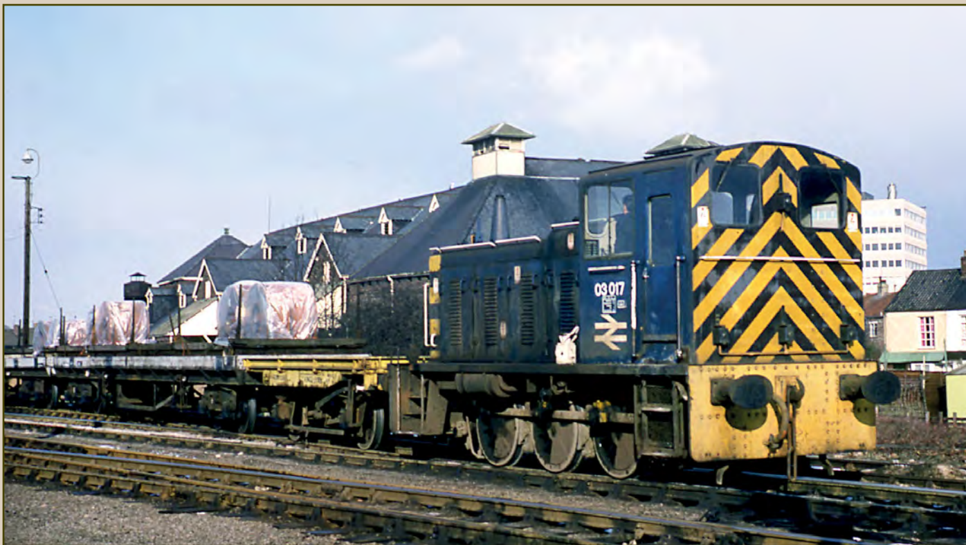
Above: The Class 03s were very popular in East Anglia, working in such locations as Ipswich, Norwich and Kings Lynn. In April 1978, No. 03017 is seen from its cab end at Kings Lynn, a loco still retaining its conical exhaust. www.colour-rail.com
